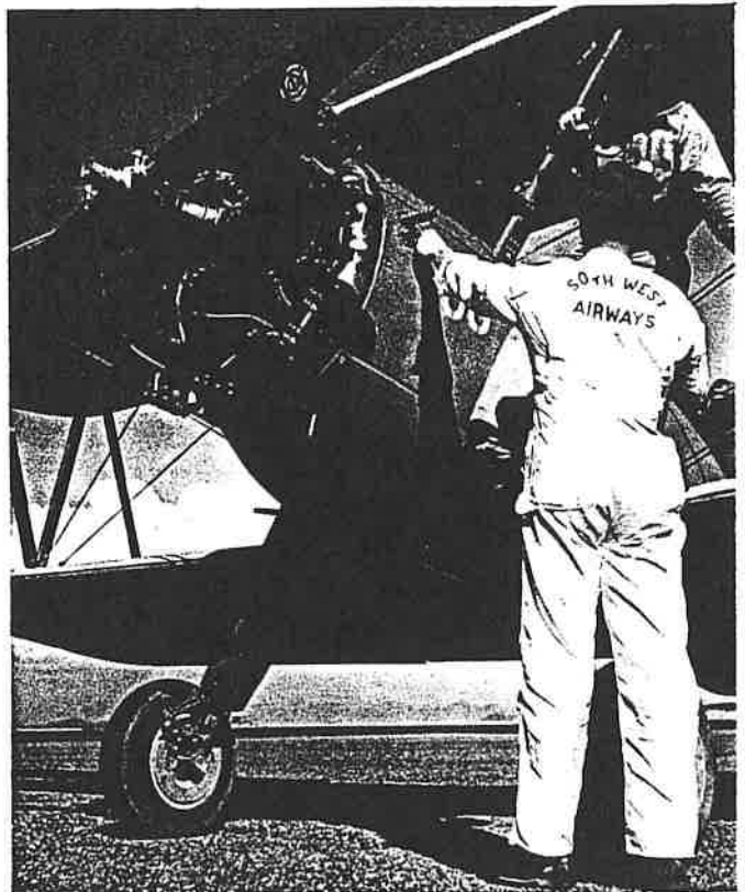
Cranking up a Continental R-670. Cranking operations were usually handled by a line crew of Pima Indians. It took brawn to start engines under the hot Arizona sun. (Southwest Airways Photo)
